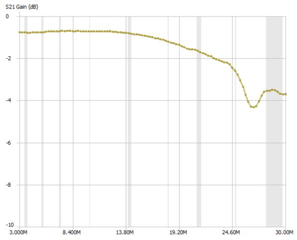
The actual loss for each transformer is half of the value shown here, so 1 dB or less up to the 15m band and less than 2 dB for the 12m and 10m bands. I'm thinking of trying different capacitors or winding styles to see if I can improve the performance for the higher bands.
